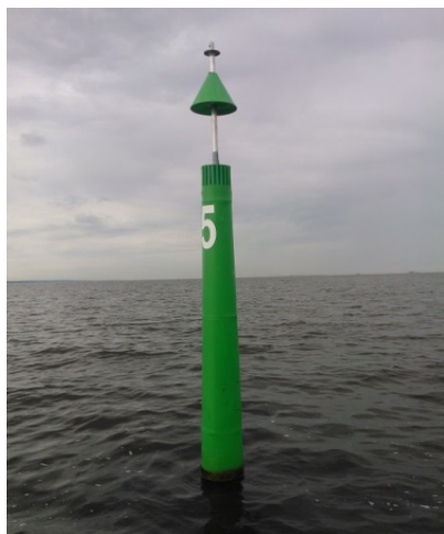
LED lantern ФСН-03МР-М with stand-alone power supply on buoy Nr. 5 (type 400/6) at approach channel of Marine Residence of the President of the Russian Federation
